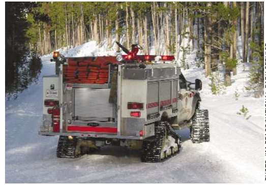
The rear hosebed carries large diameter hose and a 2½" attack line.
