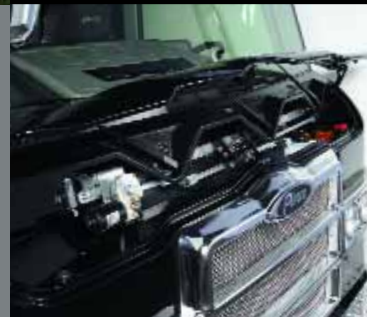
Fast access service tilt front hood
