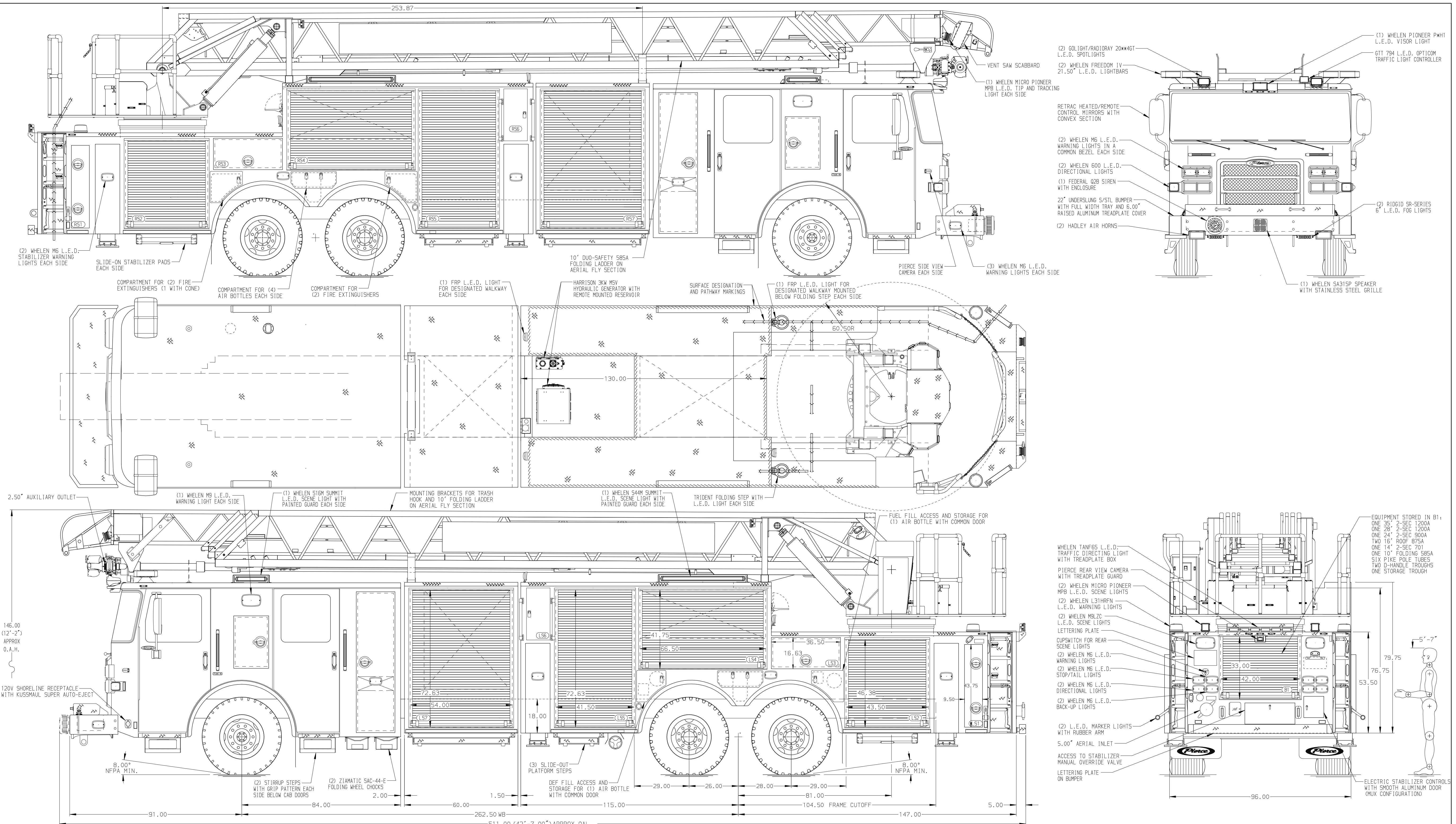
ALUMINUM BODY SIDE ROLL PROTECTION (MAXIMUM O.A.L. = 42'-7.00" (511.00")) (MAXIMUM O.A.H. = 12'-2.00" (146.00"))
