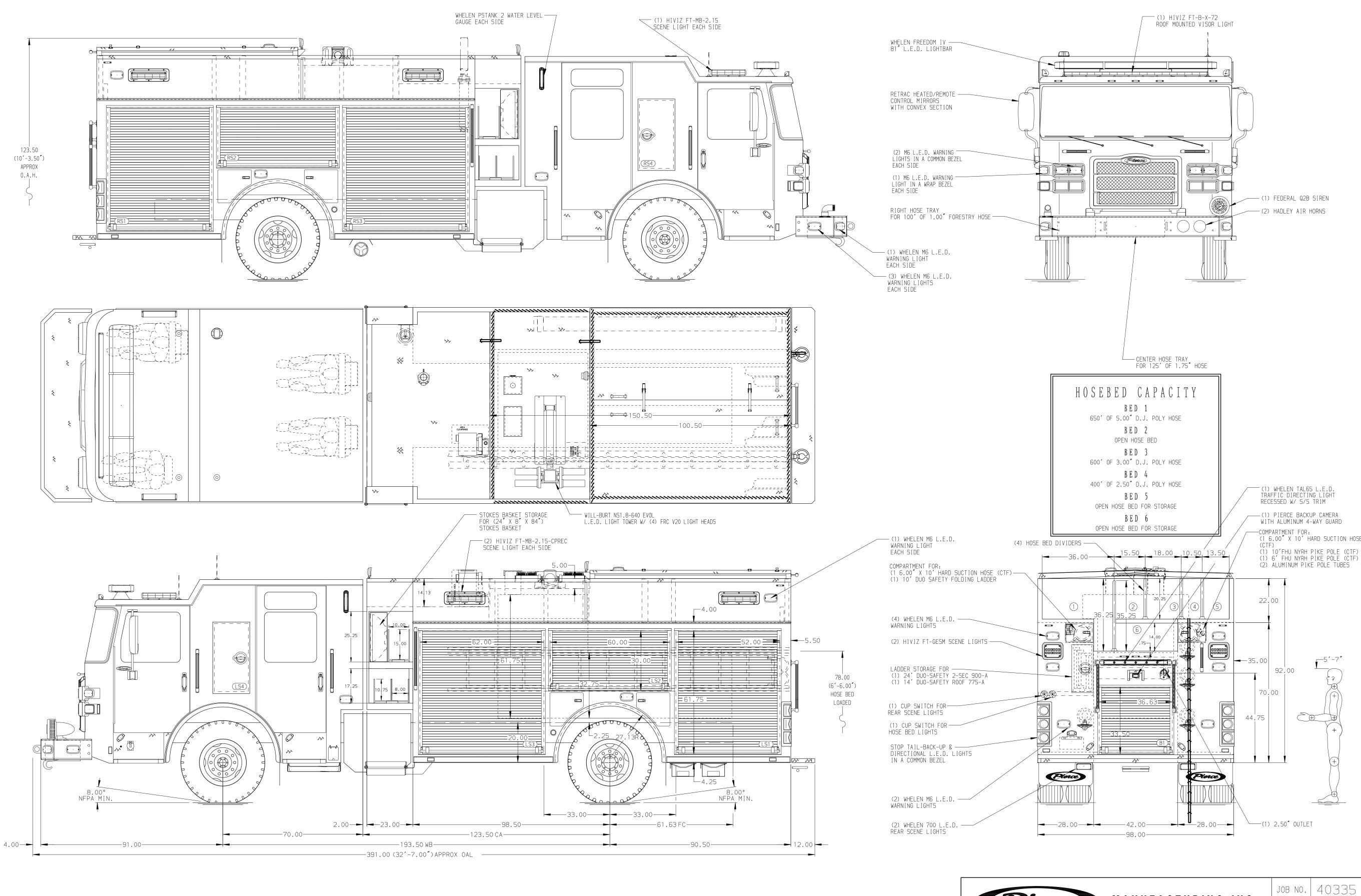
MANUFACTURING INC. SCALE DATE 1:24 DRAWN BY Pierce Pumper Approval Drawing CHASSIS 08JUL24 LST DATA MAKE CHECKED BY 7 | 17FEB25 | LST | GKH Kootenai County Fire and Rescue 09JUL24 MMF PIERCE ₿/ |230CT24 | LST | GKH SHEET SIZE SHEET NO. MODEL A 18SEP24 LST GKH DWG 40335AD REV DATE BY CH ENFROCER NO.
